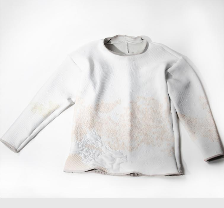
15 **Dye Test, 001:** Applied phasechanging pigment, suspended in an earlier version of the silicon mixture. Applied on 100% cotton knit. Left in vapor chamber for twelve minutes.
