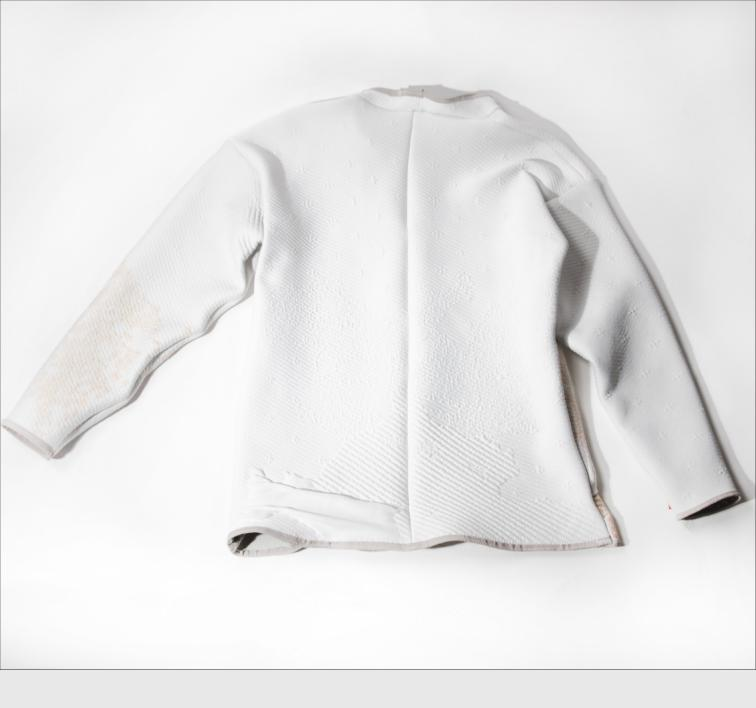
16 **Dye Test, 002:** Applied phasechanging pigment, suspended in an earlier version of the silicon mixture. Applied on 100% cotton knit.
