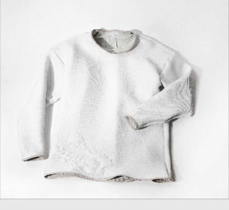
14 **Dye Test, 000:** Applied phasechanging pigment, suspended in an earlier version of the silicon mixture. Applied on 100% cotton knit.
