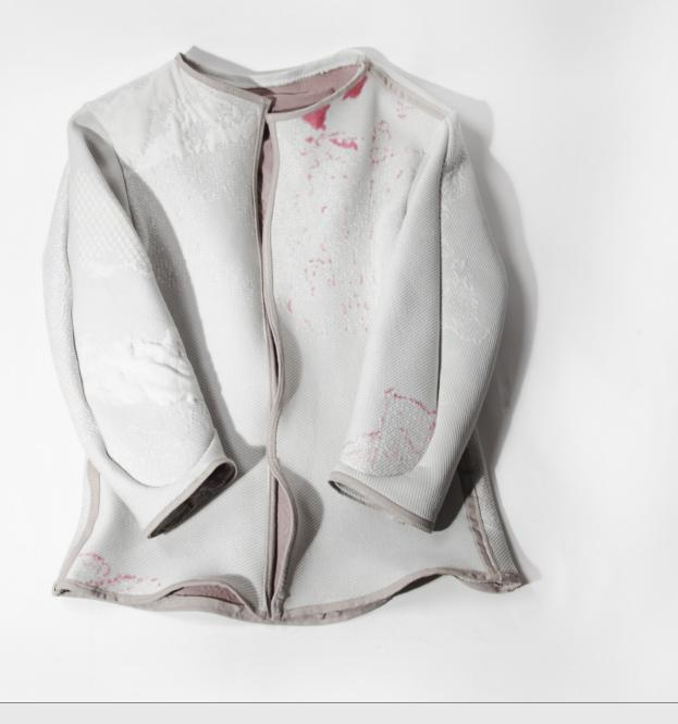
19 **Dye Test, 005:** Applied phasechanging pigment, suspended in an earlier version of the silicon mixture. Applied on 100% cotton knit. Left in vapor chamber for twelve minutes.
