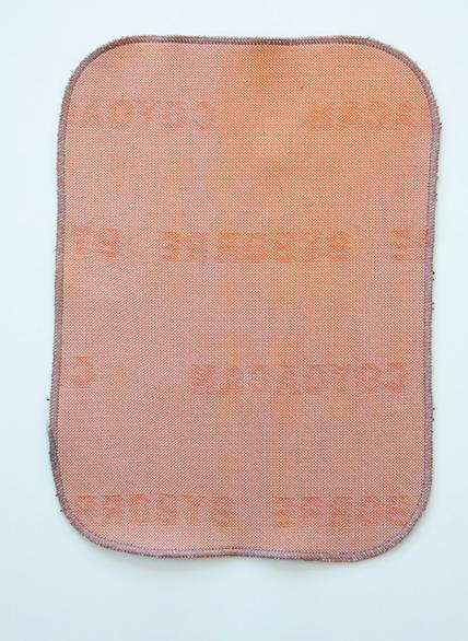
09 **Series of Dye Test, 003:** Applied phase-changing pigment directly on material sample of 40% recycled polyester and 60% cotton knit. Left in vapor chamber for four minutes.
