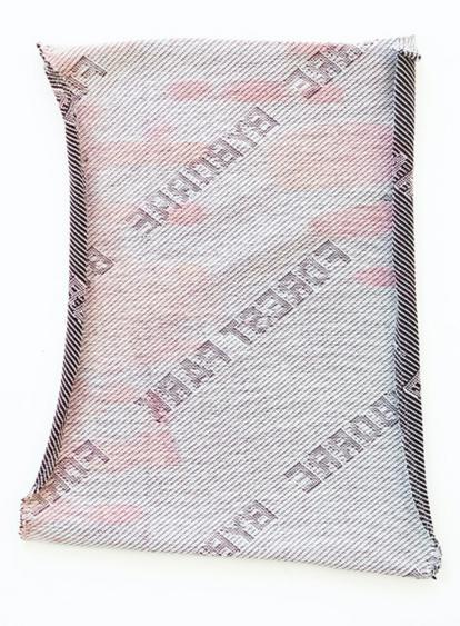
Series of Dye Test, 004: Applied phase-changing pigment directly on material sample of 55% recycled polyester, 40% cotton knit, 5% elastine. Left in vapor chamber for nine minutes.
