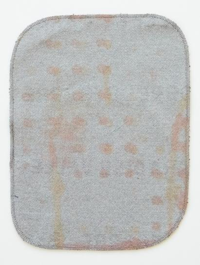
08 Series of Dye Test, 002: Applied phase-changing pigment, suspended in an earlier version of the silicon mixture. Printed via screen-printing on 100% cotton knit. Left in vapor chamber for twelve minutes.
