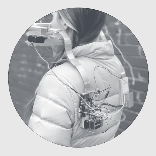
A physical computing pack, disclosed on the back of the 'helmet'. The system depends on serial communication between the air-quality sensor and two servo motors acting as the arm that opens and closes the shield. Boolean logic is used to assign values to the air-quality to tell the servo motors to stay 'open', or 'close'.
