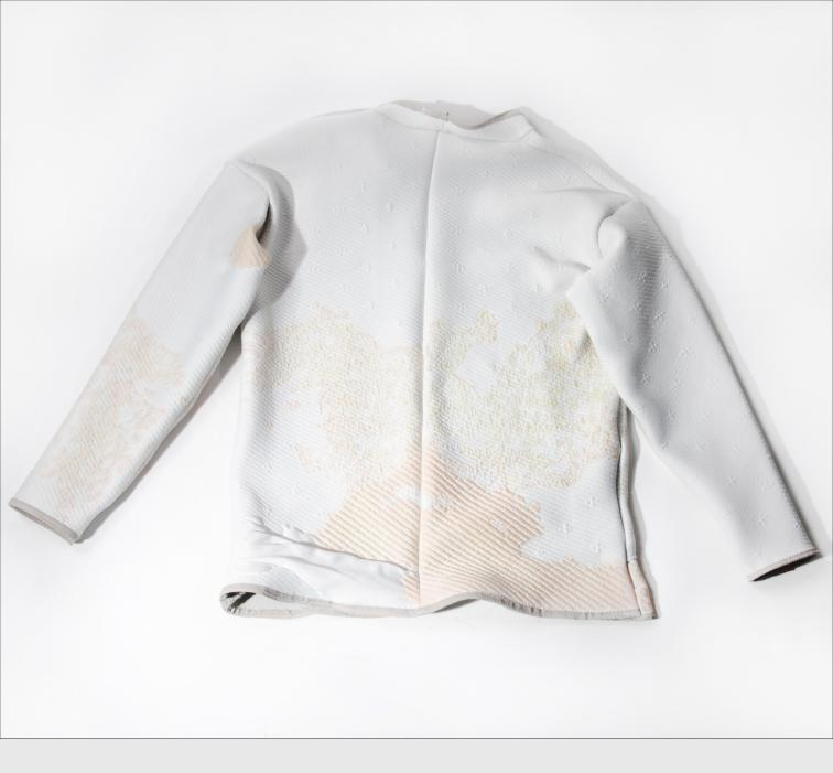
17 **Dye Test, 003:** Applied phasechanging pigment, suspended in an earlier version of the silicon mixture. Applied on 100% cotton knit. Left in vapor chamber for twelve minutes.
