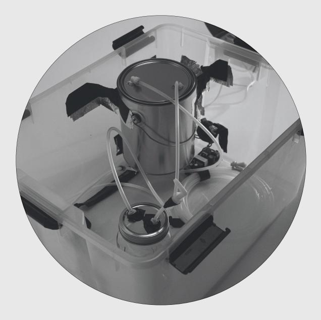
e2 A vapor chamber to carryout controlled ammonia tests. In a way, this was to falsify inputs and generate a consistent color output, and to better understand the spectrum of colors that are achieved from the phase changing pigment.
