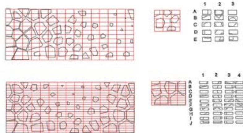
**This page: Voronoi Wall** Here, I used the voronoi in combination with the point-attract command and experimented with breaking the result apart into different potential courses of brick. I eventually settled on a set of 12 to 3D print and test.
