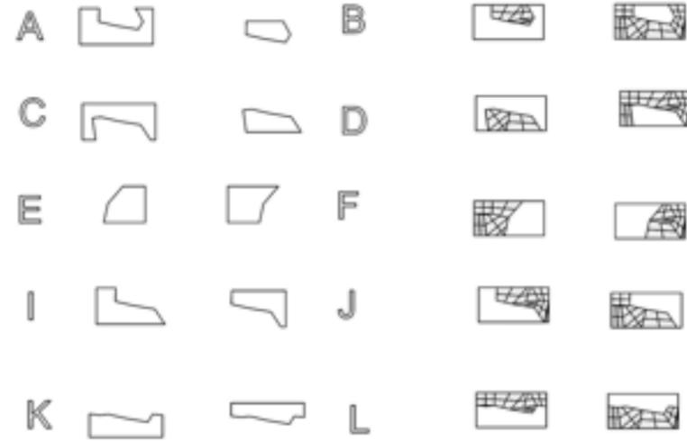
meant to represent a portion of, so I added back in what would be the boundary of the brick form, and developed a series of 10 shapes—the second 5, being the mirror shape of the first 5—and filled in the remainder of each of those shapes with my original 8 pieces, which resulted in 10 bricks that were (in different proportions) void and solid, but which any of these smaller pieces could break from in order to change the shape and directionality of the wall.
