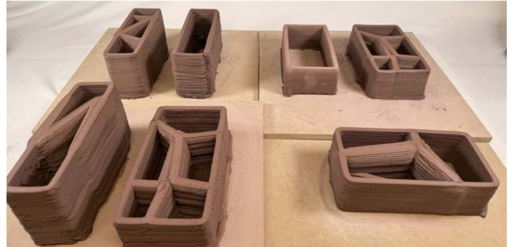
**This page: 3D Ceramic Prints of Voronoi Bricks** In these initial tests, I printed both 2.25" x 8" bricks and 4" x 8" bricks, using different numbers of points. This was an opportunity to consider which combination would give me the most compressive strength.
