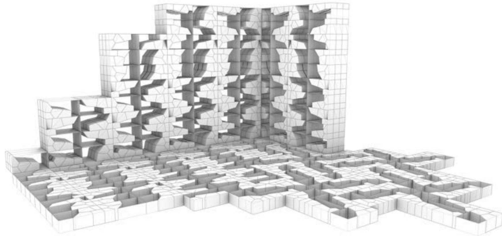
**This page: Installation Mockup.** This mockup of my installation illustrates how the module works as part of a wall, seat, path, and patio, while also working as a breeze block, waste management strategy, and water filtration system.
