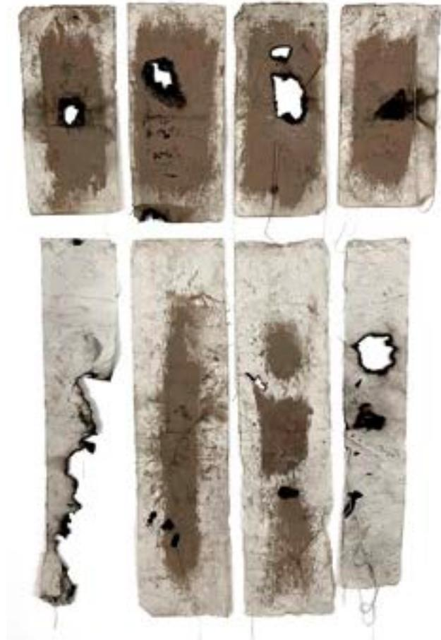
In this instance, the fabric was immersed in water and employed for manipulating the clay in the vessel production. Thus, before exposing it to the elevated temperatures of the molten glass, the fabric retained a thin layer of clay and remained moist. This imparted a certain resistance to the process, enabling it to capture some of the particles released during the extinguishing of the vessel. The moisture in the fabric also notably decelerated the explosion process.
