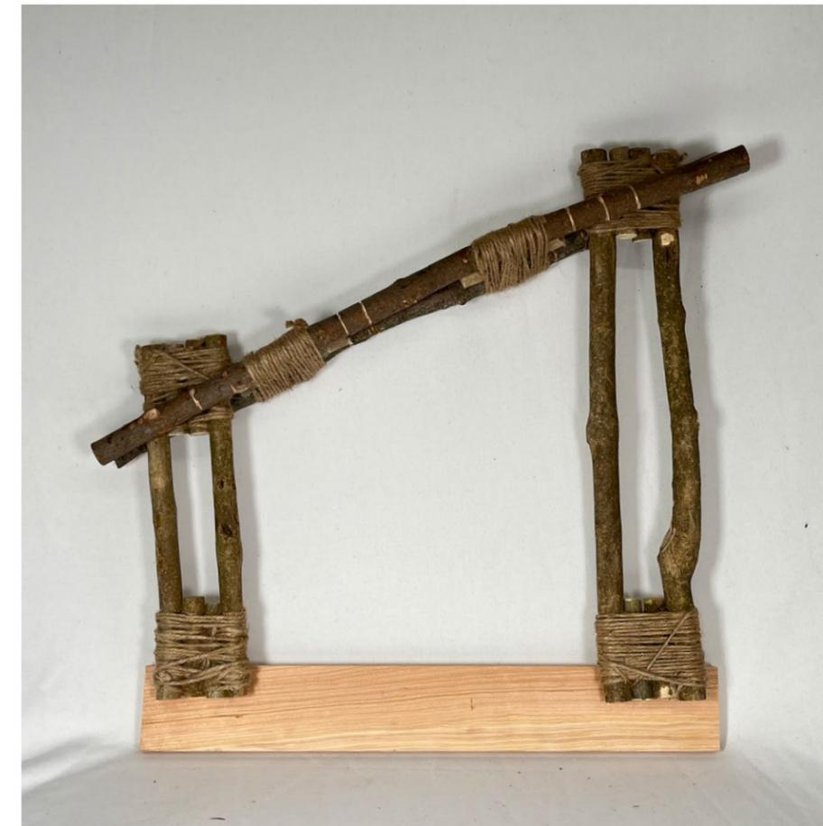
In the full-scale prototyping process, a wooden base is built to provide the foundation for the wooden sticks, which mimics the relationship between the soil and the wooden sticks. During the building of the wooden structure, the architect Anna Heringer's work METI Handmade School is referenced for the structural details, and further adjustment is applied to provide more space for the straw clay input.
