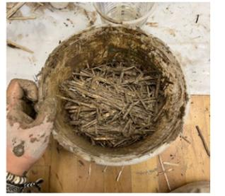
The 1:1, 1:3, and 1:6 earth-to-fiber ratios are chosen to use as the input of the three small mock-up wattle frames, these three mock-ups are built to test the permeability of the frames for water management in different site situations.
