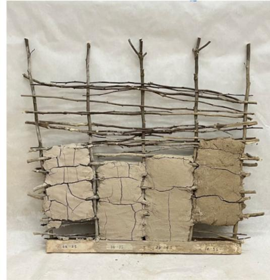
Mixture Ratio Testing (Left to right, Kaolin to Soil)
