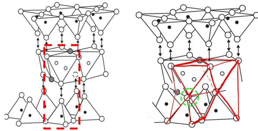
Figure 24. Left: Three-dimensional assembly of tetrahedral and octahedral sheets and formation of the 1:1 layer and the 2:1 layer. Large white circles are oxygens, large grey circles are hydroxyls, small white circles are octahedral ions and small black circles are tetrahedral ions. The image is from G.E. Christidis (2011). Right: Author's sketch
