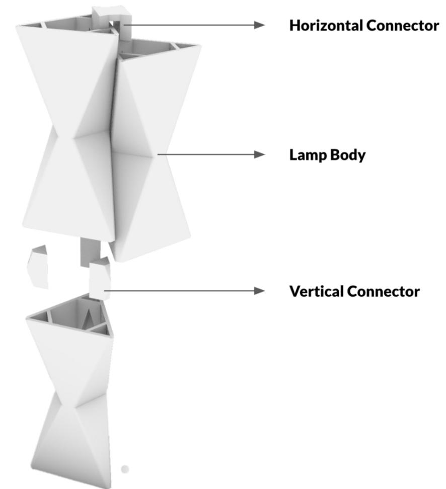
Figure 25. The connection of the modular lamp
