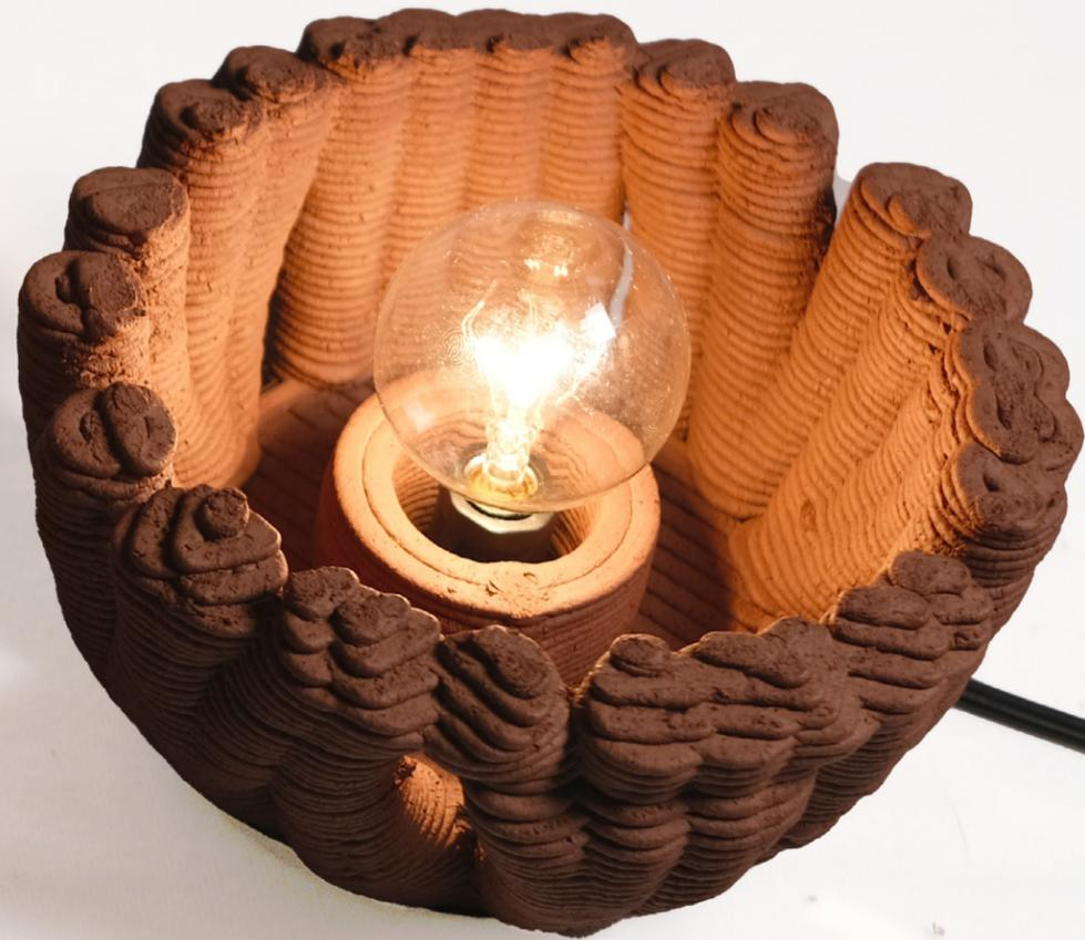
100% brick. Its characteristics are completely different from clay. It lacks plasticity and is not suitable to print for the complex modeling of 3D models.
