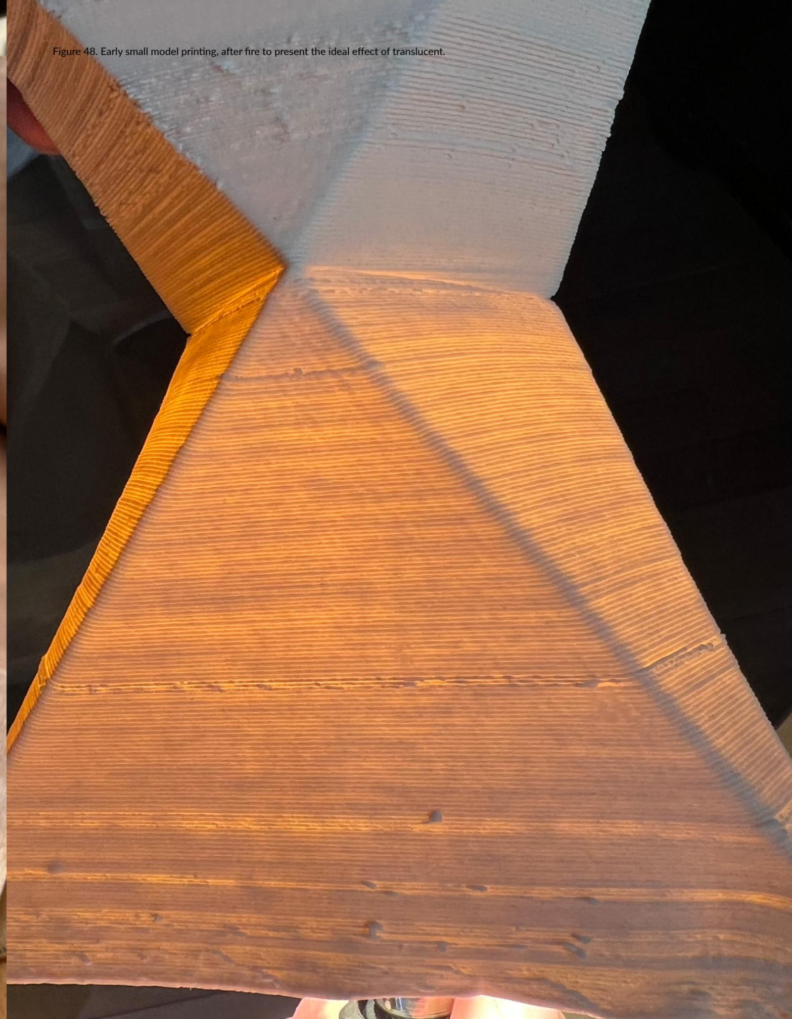
Figure 49. Printing with brick dust and alginate recipe. Due to inadequate control of the moisture content in the materials, the high moisture content caused the collapse of the entire model after the print.
