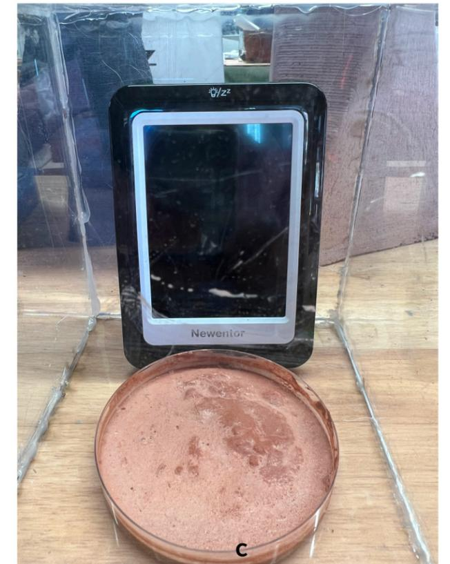
Figure 15. A: Initial carbon dioxide content 429 PPM. B: Carbon dioxide content after three hours: 400 PPM. C: Carbon dioxide content after three days: 400 PPM. Through comparison of the images, it can also be observed that the color of the samples changes over time. Upon closer examination of the image B, a transparent film can be seen forming on the surface of the sample.
