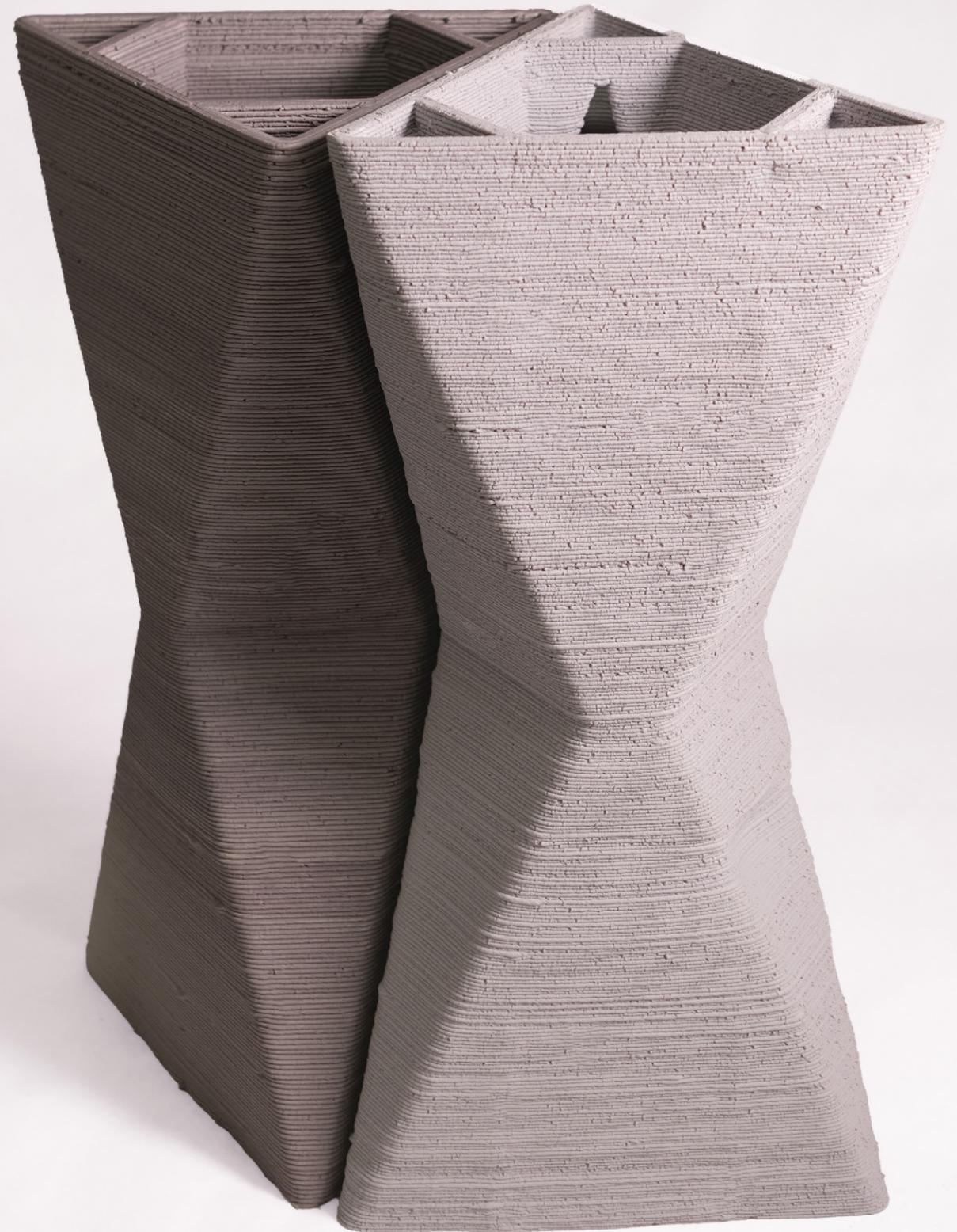
Figure 30. The initial model. However, during printing, there were inconsistencies on the upper part, resulting in the texture depicted in the image. It is fired and made of Porcelain Moist Clay and brick dust.
