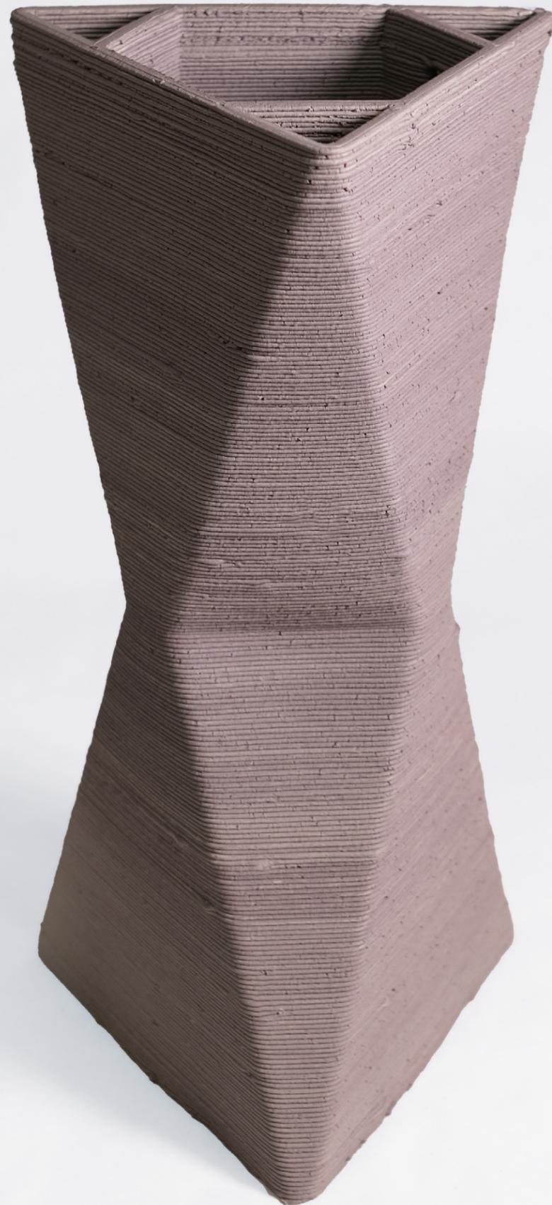
Figure 29. The initial two models stack horizontally. These two models are made of the same materials. However, the color looks different. It is because the drying time is different.
