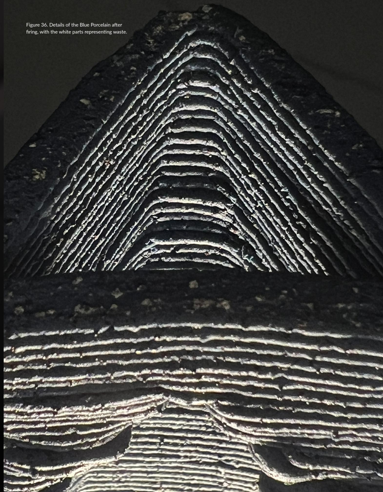
Figure 37. Close-up detail image. After firing, the tile dust changes from brown-yellow to black.
