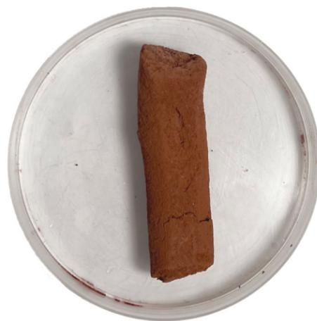
Figure 43. Brick+Casein recipe is extruded from the 3D printer.
